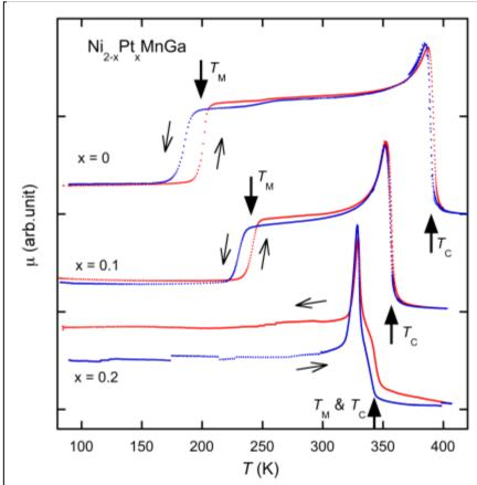
Temperature dependence of the permeability of the Ferromagnetic Shape Memory Alloys  $Ni_{2-x}Pt_xMnGa$  (x= 0, 0.1, 0.2).  $T_M$ 's (martensitic transition temperature) are increased and  $T_C$ 's (Curie temperature) are decreased with the Pt substitution, x.
