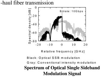
(1) Optical single sideband (SSB) modulation for long
