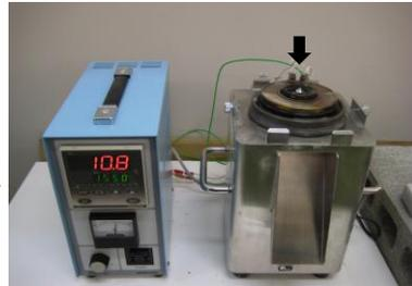
Developed Milling Machine(lab. scale)
