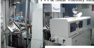
Using ca.50 g materials  $\Rightarrow$  Measuring for Process-ability and flow-ability Solidification, Rheology, thermal properties etc.
