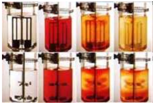
Effect of impeller shape on mixing efficiency.
