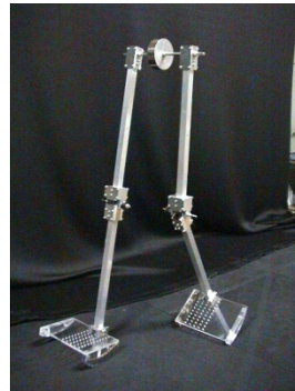
Passive dynamic walking mechanism
